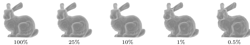
Figure 11: Rendered Bunny meshes for the partitioned_batch implementation with 16 threads at target vertex percentages 100%, 25%, 10%, 1%, and 0.5%.
