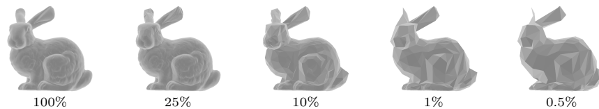
Figure 12: Rendered Bunny meshes for the partitioned_batch_boundary implementation with 16 threads at target vertex percentages 100%, 25%, 10%, 1%, and 0.5%.
